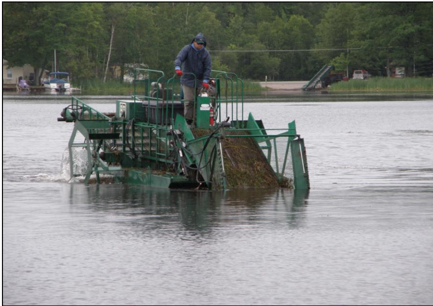
Figure 54. A mechanical harvester. Photo courtesy of Dave Foley.
