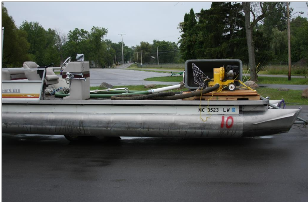
Figure 55. A DASH boat for hand-removal of watermilfoil or other nuisance vegetation.
