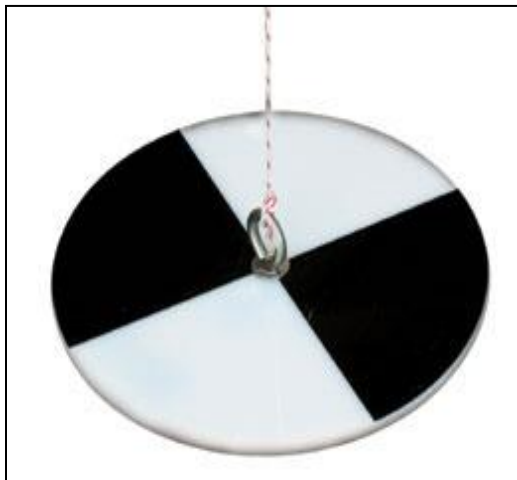
Figure 18. A Secchi disk
